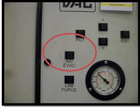
A photograph of a control panel with various buttons and a gauge. A red circle highlights the 'A/C EVAC' button. |
